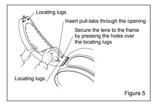
**9.1.1.6** Secure the lenses to the frame by pressing the lens mounting holes on the pull-tab end of the lenses onto the mushroom-shaped locating lugs. The slots on the other end of the lenses fit over the locating lugs on the latch end of the frame.
