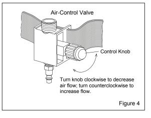
**6.2.1** Clemco's ACV air-control valve allows the user to increase or decrease the volume of breathing-air while wearing the supplied-air respirator. The valve provides a range of 7 to 10 cfm of breathing-air when the respirator is supplied with respirable air as noted in Section 4.4.
