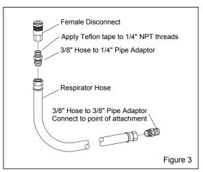
**3.4.3** Attach the adapter/disconnect assembly to one end of the respirator hose.
